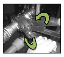
6.- Connect a hose to the drain and overflow connection located at the bottom of the water tank. Use a flexible hose with 10mm internal diameter.
