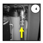
5.- Connect the outlet water hose going to the application to the 2" nipple located at the pump outlet (superplus models) or evaporator outlet (standard models). See the identification labels.
