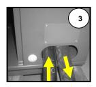
4.- Connect the inlet water hose coming from the application to the 2" nipple located at the inlet of the water filter.
